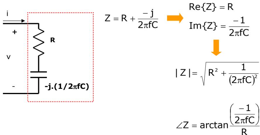
For  $R = 1 \text{ k}\Omega$  and  $C = 100 \text{ nF}$  ( $10^{-9} \text{ F}$ ) the following graphs are obtained:
