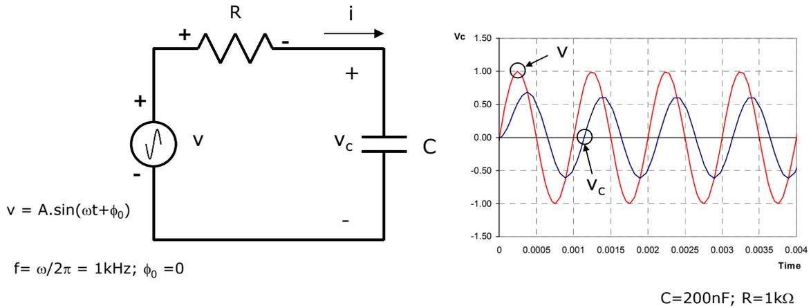
The voltage at the capacitor is a sinusoidal with the same frequency as the voltage source. The only differences are the amplitude and the phase. The same can be said about all the voltages and currents around the circuit. This is a fundamental property of linear circuits (for instance, any combination of resistors, capacitors and inductors):
