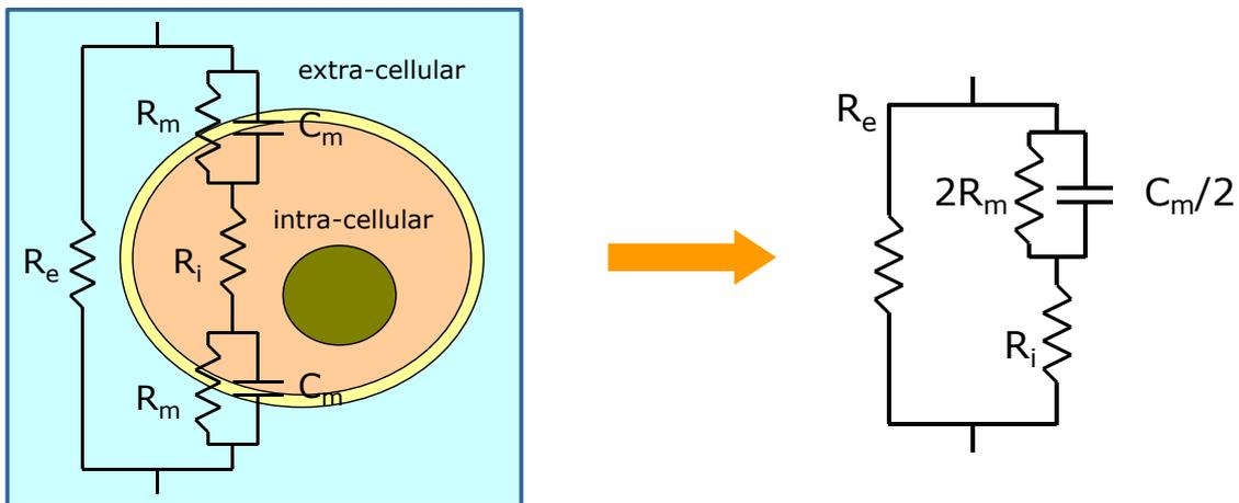
The circuit on the right is equivalent to the left model after performing some simplifications (resistances in series and capacitances in parallel). The same simplifications can be applied to reduce a tissue composed by many cells to a single cell equivalent circuit.
