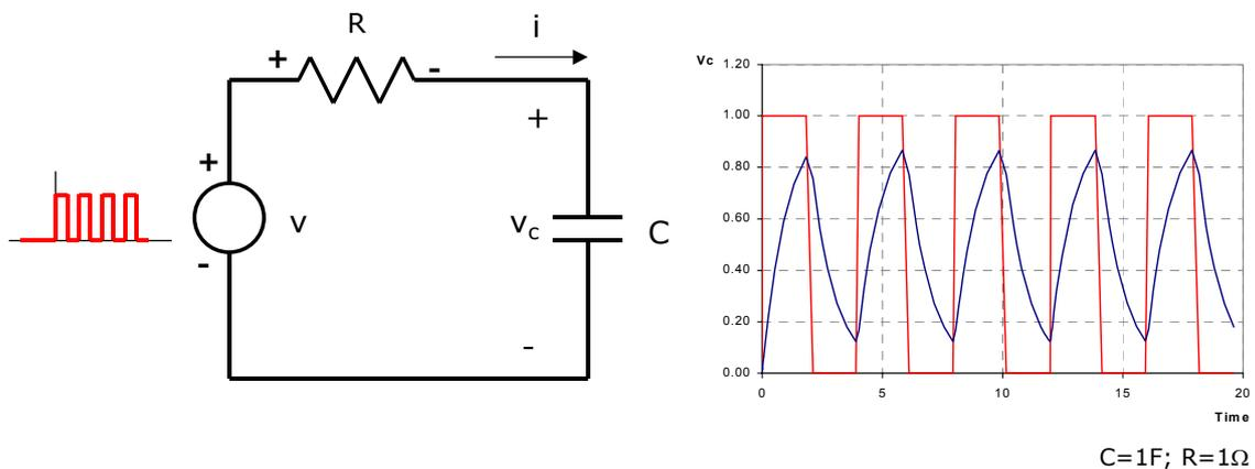
At the beginning the capacitance is discharged ( $Q=0$  Coulombs) and, consequently, the voltage difference between its terminals is 0 V. The first input voltage pulse (plotted in red) causes some current to flow through the resistance and starts to charge the capacitance. However, since the capacitance increases its voltage (plotted in blue), the current decreases and the voltage evolution is flattened.
