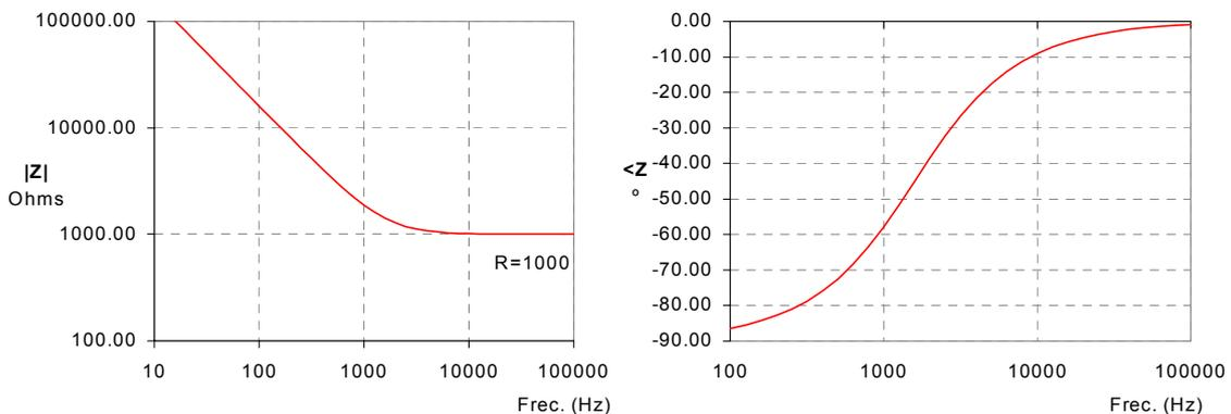
These graphs are the **Bode plots** of the impedance. On the left, the magnitude, or modulus, of the impedance is displayed for each frequency ( $f$ ). Both axes, horizontal and vertical, are expressed in logarithm base 10. The graph on the right shows the phase value for each frequency. In this case, only the frequency is expressed in the logarithm form.
