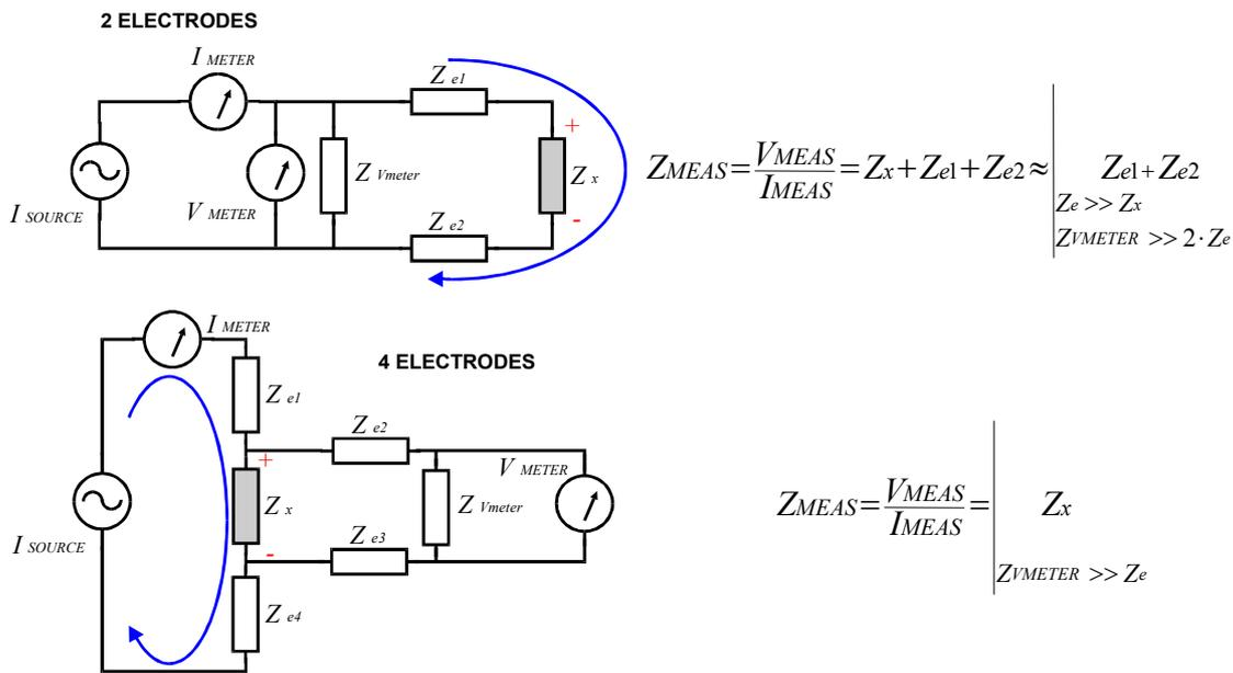
Of course, the four-electrode method is not totally free from errors. Other parasitic impedances (e.g. capacitances between wires or instrumentation input impedances) combined with the electrode-electrolyte impedances cause errors at high and low frequencies (Pallás-Areny et Webster, 1993) and that constrains the useful measurement band of the four-electrode method from some Hz to hundreds of MHz.
