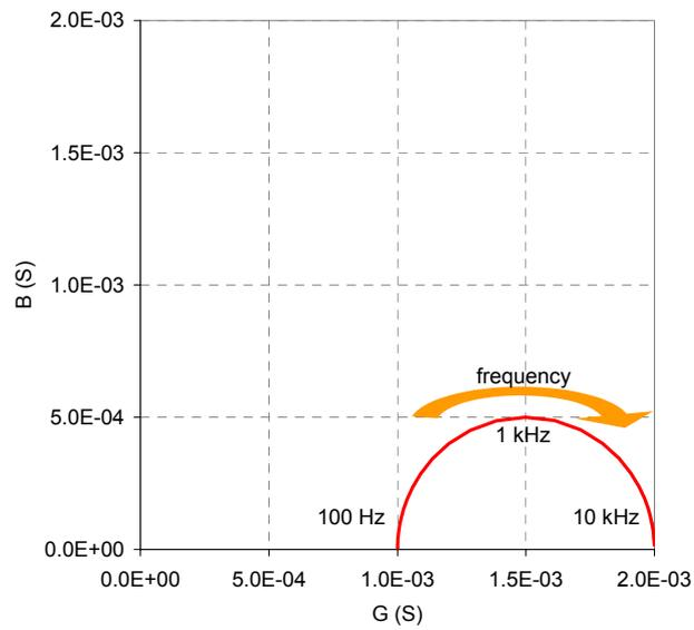
The scaling factor ( $K$ ) is  $(\pi \times 1 \text{ cm}^2)/(2 \text{ cm}) = 1.57 \text{ cm}$ . Then, the conductivity ( $\sigma = G/K$ ) and the relative permittivity ( $\epsilon_r = \epsilon/\epsilon_0$ ,  $\epsilon_0 = 8.8 \times 10^{-14} \text{ F/cm}$ ;  $\epsilon = B/(\omega K) = B/(2\pi fK)$ ) can be obtained from the conductance ( $G$ ) and susceptance ( $B$ ) values:
